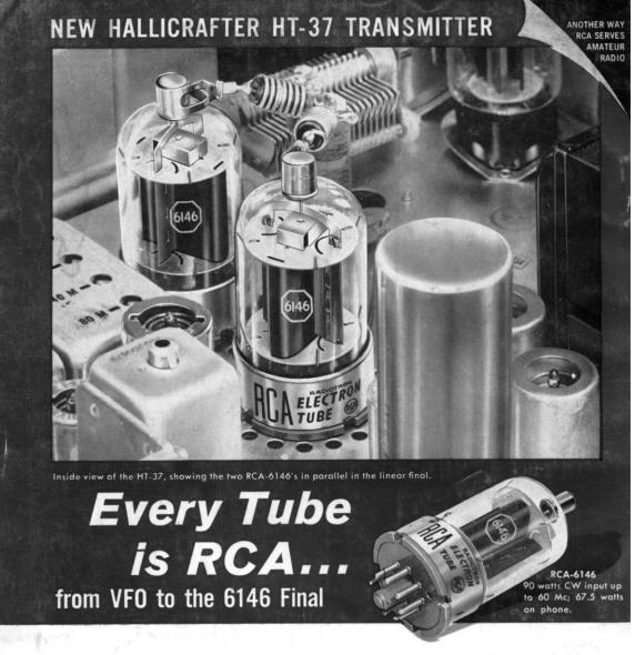
Pictured here is one of the newest, most modern SSB-AM-CW transmitters in amateur radio. It's the medium-power 10-to-80 meter HT-37. RCA is proud that Hallicrafter designers specified an RCA tube for every stage in this outstanding 18-tube rig—including the linear final!
