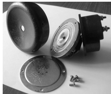
Fig 1. Low impedance cone headphone (DLR no 5)
