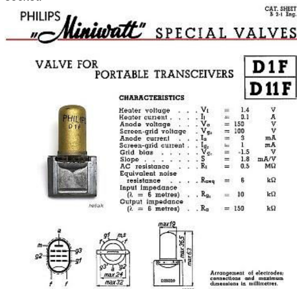
Figure 3. Edited datasheet for the D1F valve [7]
