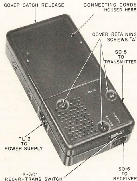
Figure 10. Filter-Accessory Unit RA-6 showing RECVR-TRANS switch.
