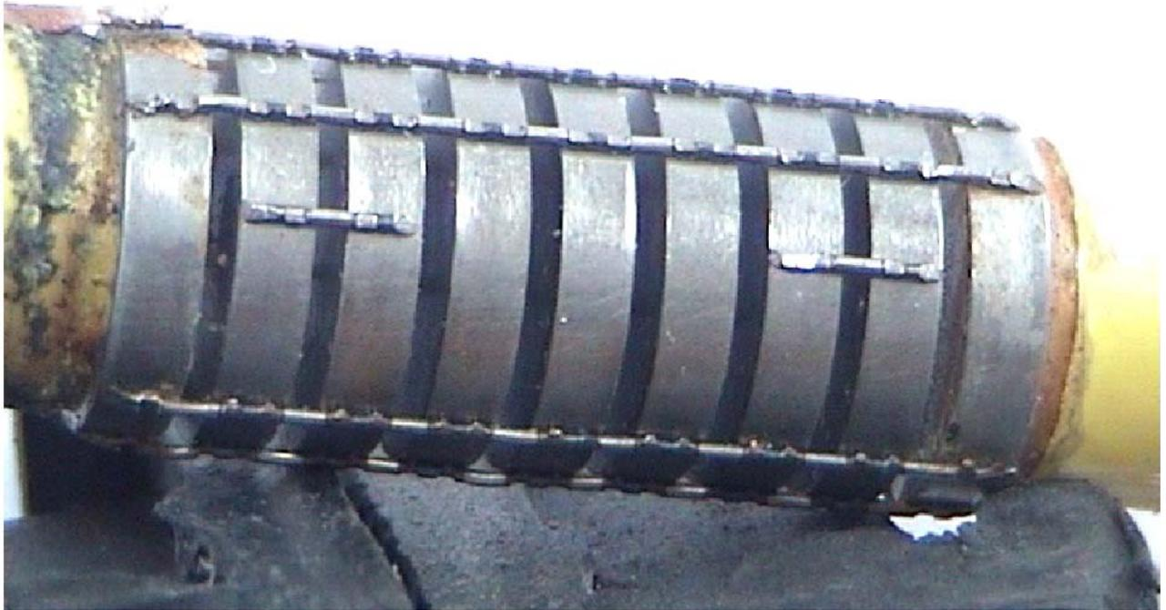
You will see that the filter comprises a set of disks with a coil at each end. This assembly will almost certainly need to be cleaned. In my case the debris from the foam had gone between the disks. Fortunately it seems to clean off quite well in alcohol.
