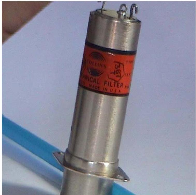
The mechanical assembly has a flat strip earth wire which is spot welded to the disk assembly, and is also trapped and soldered together with the end cap at the input end (nearest the flange). Once the foam has broken down, the earth wire is the only means of longitudinal constraint. There is no longer any lateral constraint and if you gently shake the filter from side to side you can probably feel the internal assembly flopping around.
