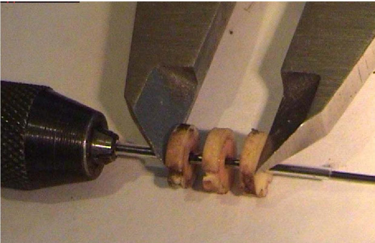
Here you see the three cheek pieces threaded onto the PTFE sleeving. There is a length of blue pivot steel inserted into the sleeving. The pin vice is gripping the sleeving in order to drive it. Note that the outside distance of the outer cheeks should be about 9.8mm. The centre cheek is centrally disposed between them.
