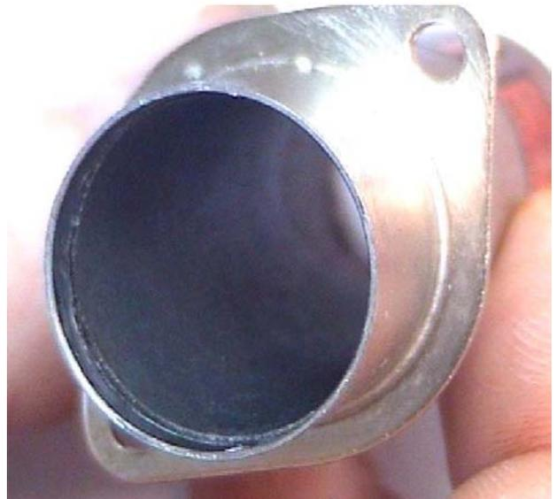
Make sure that the end caps are spotlessly clean, especially around the insulators. I placed a layer of Kapton tape over the internal surface. This was just a precaution to protect the fine wires from heat when re-soldering the case.
