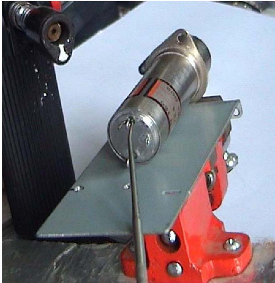
It is quite possible to do this without burning the label. Once you see the solder start to run, carefully put down the butane torch (something else I didn't do first time round) and then gently pull the cap. It should slide out with little resistance. Let it rest on the tray to cool.
