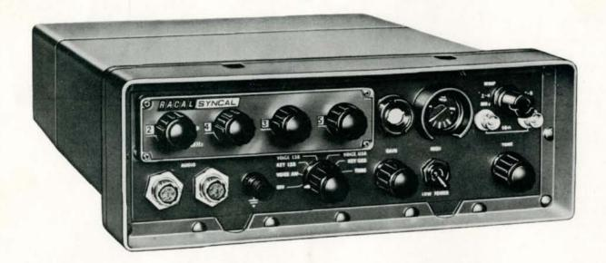
The Racal TRA.921 "Syncal" Manpack is designed for high performance, low cost, military or civil communication requirements. Providing h.f. transmission and reception in the 2 to 8 MHz frequency range, the synthesizer controlled TRA.921 is particularly suited for the manpack role, but may be used as a fixed or vehicle station by using selected ancillary items.
