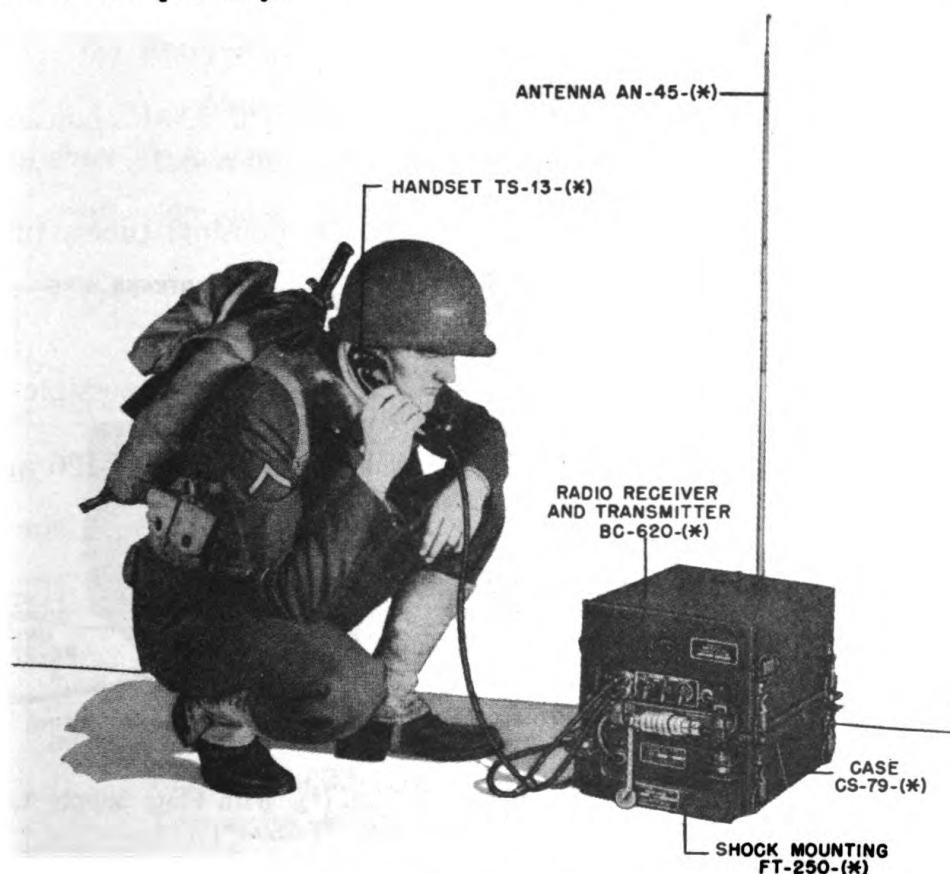
Figure 1. Radio Receiver and Transmitter BC-620-(*), With Battery Case CS-79-(*)
