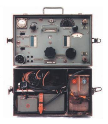
Torn.E.b with Battery Box including Vibrator EW.b
