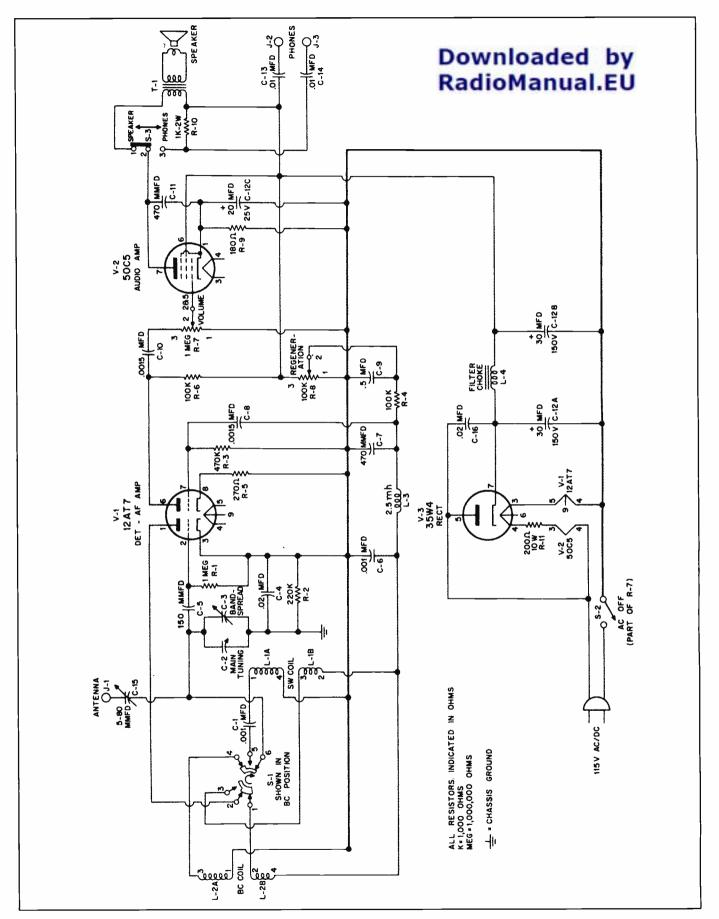
Figure 2: The Knight-kit Space Spanner schematic.
