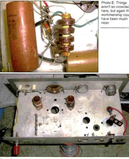
Photo F: Most of the original components couldn't be salvaged and except for a few major pieces, the chassis was stripped bare.
