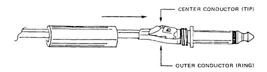
FIGURE 1-3 ATTACHING CABLE TO PHONE PLUG CONNECTOR
