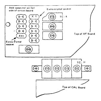
FIGURE 2-2 LOCATIONS OF EXTRA CRYSTAL AND CAPACITOR
