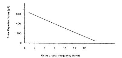
FIGURE 2-3 CHART OF EXTRA CRYSTAL FREQUENCY VS. CAPACITOR VALUE FOR 3.5 - 10 MHz RANGE
