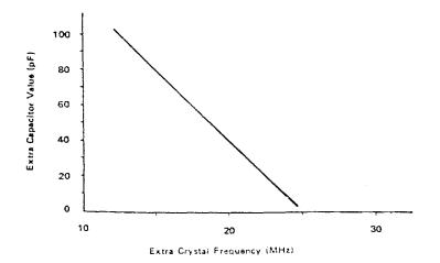
FIGURE 2-4 CHART OF EXTRA CRYSTAL FREQUENCY VS. CAPACITOR VALUE FOR 10.0 - 30 MHz
