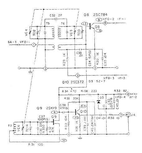
SCHEMATIC DIAGRAM OF VFO SECTION
