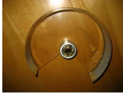
View of repaired hub that has stress cracks
