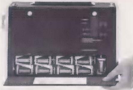
For battery operation, eight 1.5-volt mono cells are required. (Size D; international designation: R 20, e. g. Pertrix 222. Where especially long life is required, the Mallory MN 1300 is recommended). A ninth battery is used to light the dial; it does not affect operation of the receiver.
