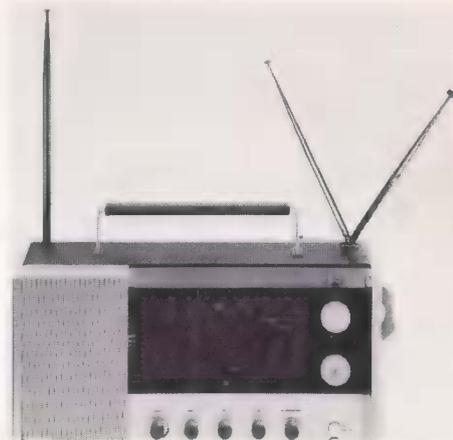
The instrument is equipped with a telescopic dipole for the FM band, a telescopic antenna for SW bands, and a ferrite antenna for LW, MW, and sw 8 bands.
