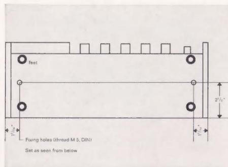
When permanently installing the receiver, insert mounting screws (M 5 thread) into the two threaded sockets at the base of the unit.
