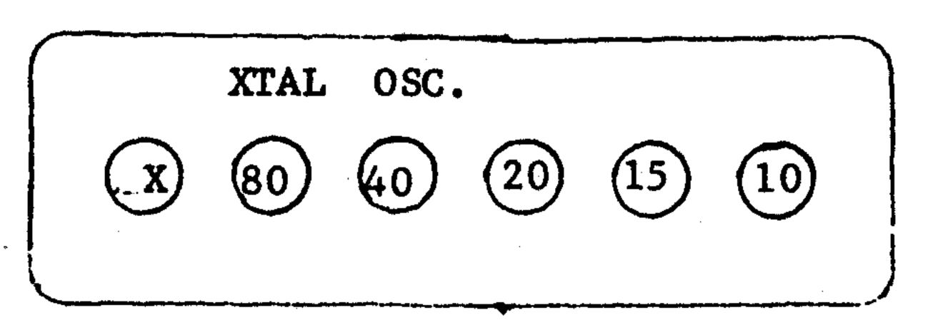
The high frequency crystal oscillator plate tuning coils should all be peaked for maximum output, consistent with proper calibration. If these are detuned too far to obtain exact calibration, the power output may drop, or the crystals may not oscillate reliably.
