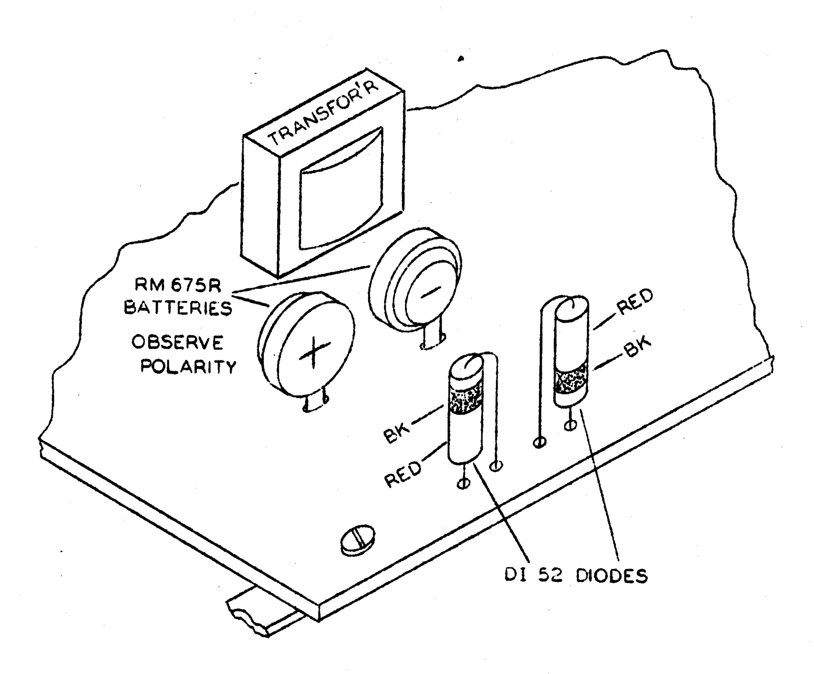
The RM400R batteries formerly used in the 100V audio limiter have been replaced with the RM675R. As you will note in the sketch above, the polarity of the RM675R is opposite to that of the RM400R, shown in the 100V manual. Be careful to install the batteries in the manner shown above.
