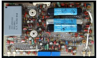
Figure 9 - IF Mechanical Filter Board
