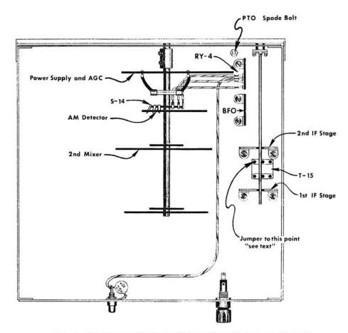
RY-4 CIRCUIT BOARD INSTALLATION DIAGRAM
