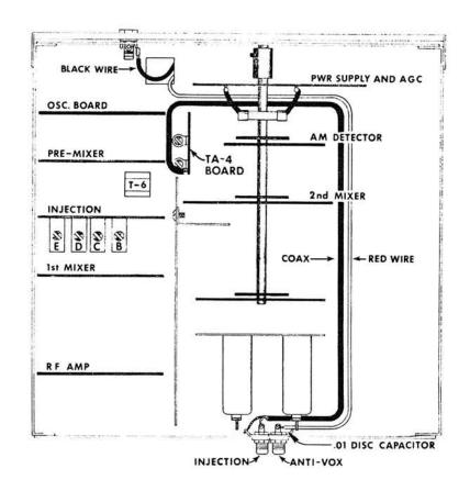
TA-4 CIRCUIT BOARD INSTALLATION DIAGRAM Figure
