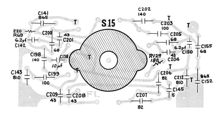
50 kHz FILTER CIRCUIT BOARD Figure 34
