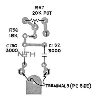
T-NOTCH FILTER CIRCUIT BOARD Figure 33
