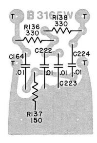
PARALLEL BRIDGE T-NOTCH FILTER CIRCUIT BOARD Figure 39
