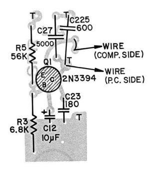
LOOP ANTENNA CIRCUIT BOARD Figure 22
