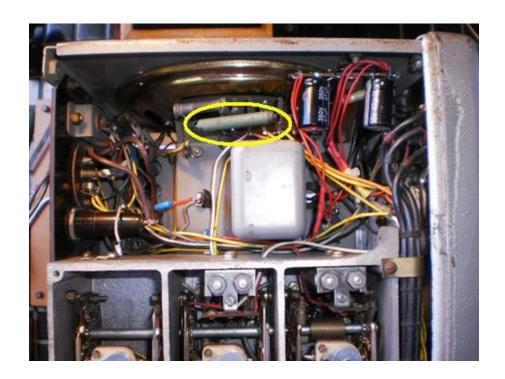
Some tuning and electrolytic (cathode decoupling) capacitors were replaced.
