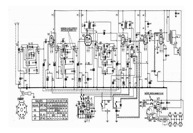
The seven valves are Rimlock types which have an edge guide cast into their glass bases. They are; 3 tubes **UAF 42** ( RF , IF , Detector , Audio ) , a **UCH42** ( Oscillator / Mixer) , a **UL41** (Output ) and a **UY41** ( rectifier ) .
