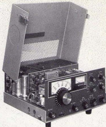
The FPM-300 offers unusual flexibility for mobile installation and removal because of its flip-up hinged cover and chassis. Hinged design permits quick and easy access to internal adjustments without disassembly.
