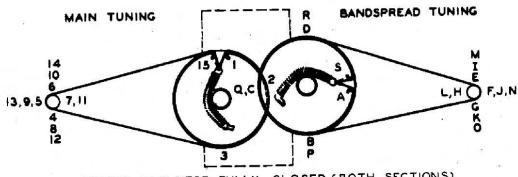
TUNING CAPACITOR FULLY CLOSED (BOTH SECTIONS).
