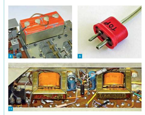
Unlike the GC-1A, which has a momentary action dial lamp switch when battery power is in use, the UK Mohican has a normal on/off type. The original dial lamps are rated 6.3V 110mA. They are connected in series with a 12 $\Omega$  resistor and this chain draws about 100mA from a 12V supply, more than the quiescent current drain of the receiver itself. This can be greatly reduced by replacing the lamps by a pair of LEDs with an appropriately larger value of series resistor.
