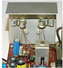
Fig. 8: Unlike the US Mohican, the GC-1U accommodates a pair of 6V PP1 batteries. Fig. 9: A polarised plug is used for connecting an external power supply. Fig. 10: Higher power audio output transistors can be mounted on an extended heatsink. Fig. 11: An output transformer (right) for a larger 3 $\Omega$  loudspeaker can be fitted under the chassis.
