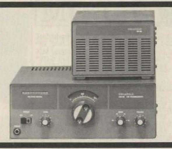
nter Heath's latest Novice transceiver, the HW-99, complete with an integral power supply and a solid 50 Watts on 10, 15, 40, and 80 meters. The rig is solid state and ruggedly designed, and should see years of trouble-free service. The minimal controls will simplify life for the Novice, but will utterly frustrate just about anyone else.
