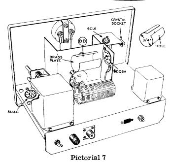
break loose the brass neutralizing plate when sliding the tube into the plate.
