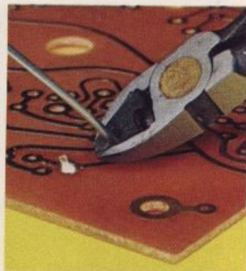
CLIP OFF THE EXCESS WIRE LENGTH.
