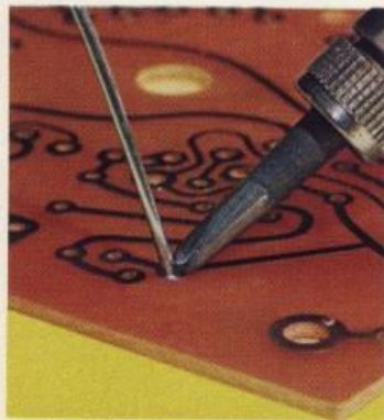
HEAT BOTH WIRE AND FOIL.
