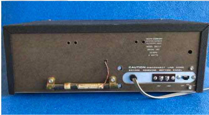
Figure 2: SW-717 General Coverage Receiver Rear view showing ferrite AM band antenna.
