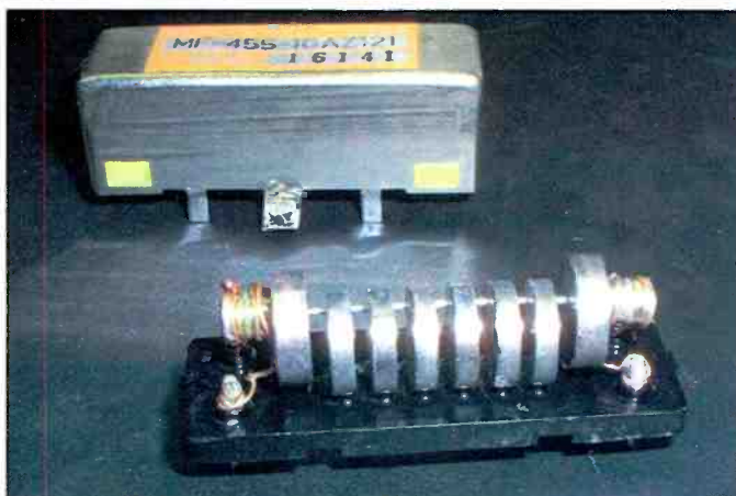
Photo 4: After using a solvent to melt away the old foam rubber, followed by several rinses in pure isopropyl alcohol, the old filter is free of contamination.
