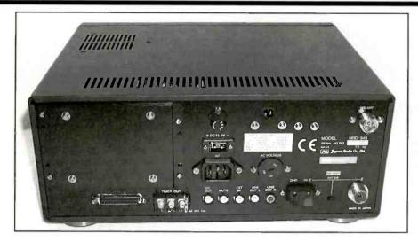
Lots of connections are available on the back panel. Note the N type connector at the upper right for the wideband converter option. HF antennas are connected at the lower right either with a PL-259 coaxial connector, or wires. I also thought it was interesting that JRC uses a DB-25 connector for the serial port instead of the more common DB-9. You'll need a null modem adapter or cable to connect to the computer correctly.
