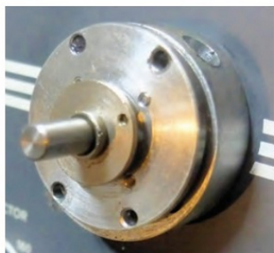
PHOTO 5: The reduction drive and spacer.
