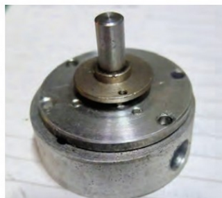
PHOTO 4: Reduction drive as removed.
