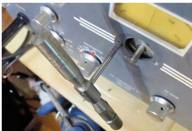
PHOTO 8: Tapping the front panel M5.
