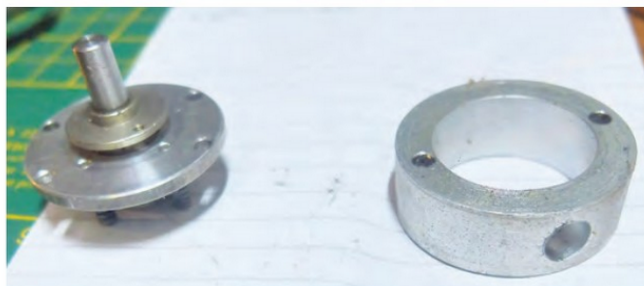
PHOTO 6: The drive and spacer separated.
