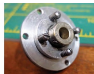
PHOTO 9: The clutch drive 'up close'.
