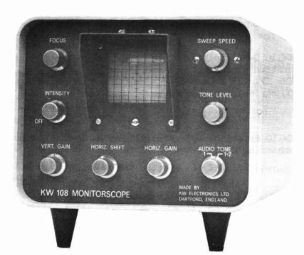
The KW108 "Monitorscope" is a convenient instrument allowing "on-the-air" monitoring and testing of an amateur radio transmission on all bands from 160M through 10M.
