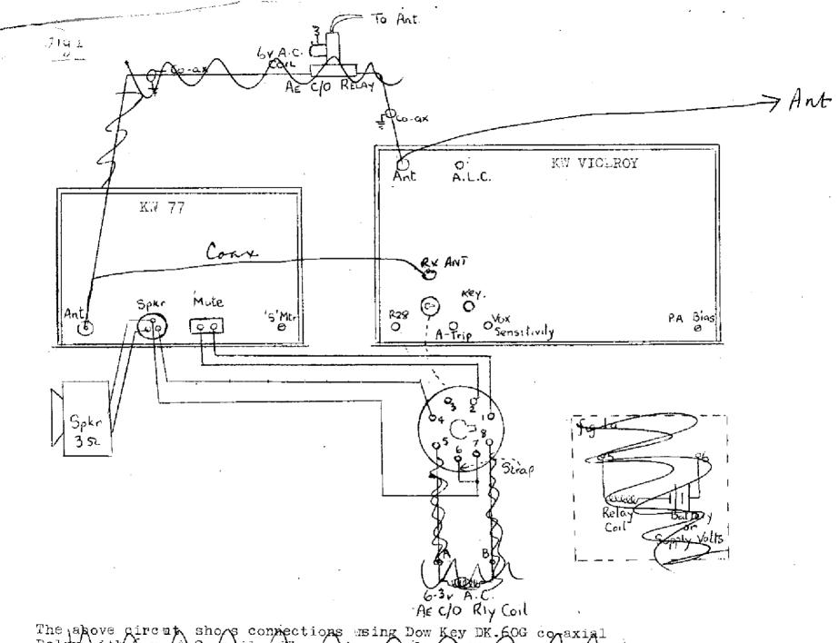
The above circut shows connections using Dow Key DK.60G co axial Relay ith 6 v. A C. coil. Then using an alternative Relay and external Fower Supply for the relay use plans 5 & 6 connected as shown in fig. 1a
