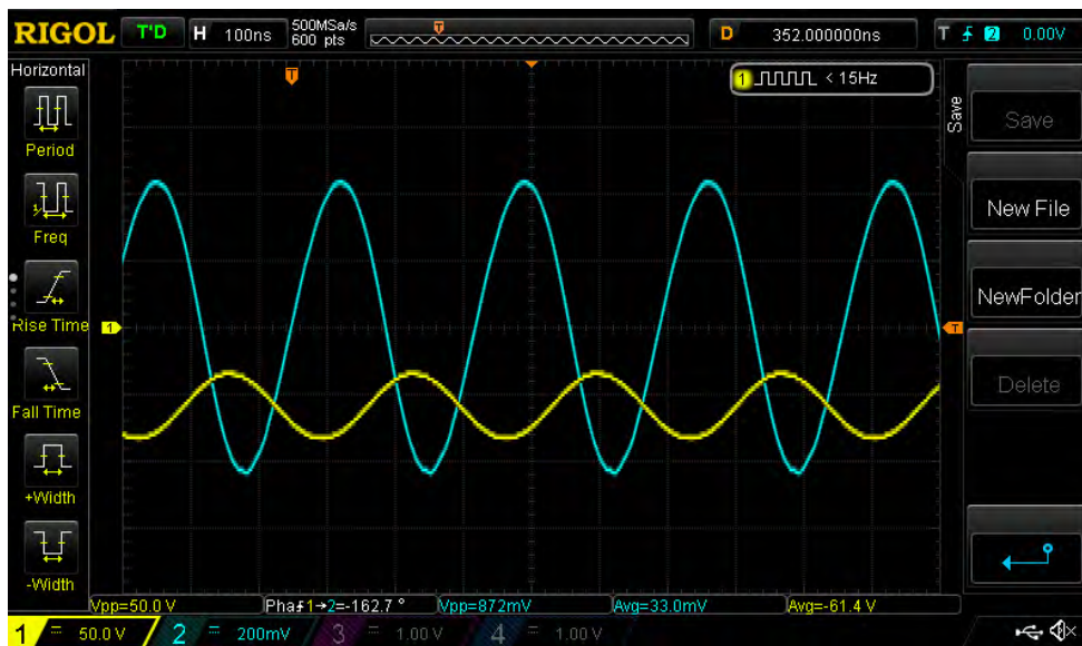
Figure 12 80 metres PA grid voltage DC coupled in yellow and driver grid voltage AC coupled in blue. Why was there grid current being drawn when the PA grid voltage was nowhere near zero?
