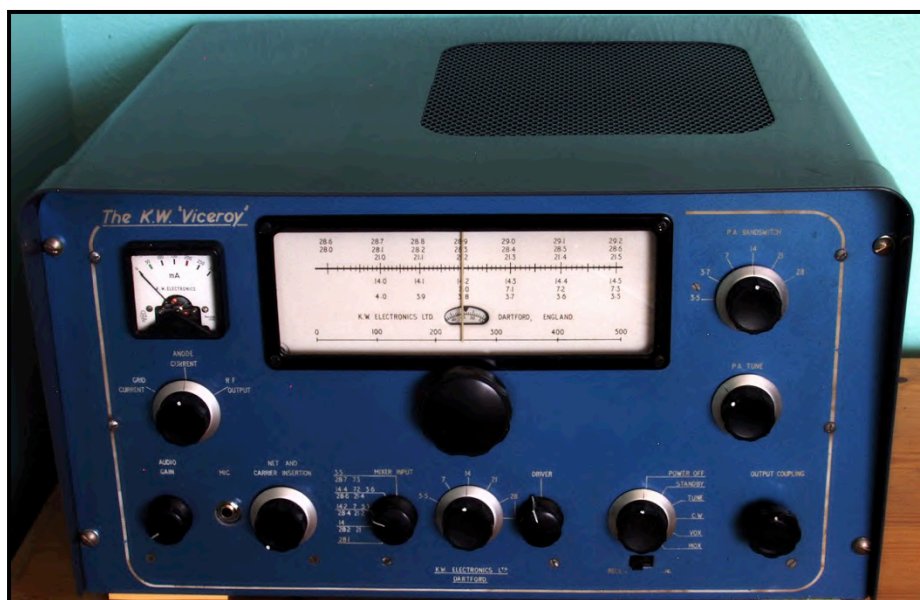
Figure 11. The restored Viceroy Mk IV with the original front panel and its powder-coated case.
