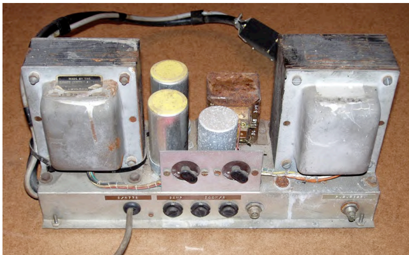
Figure 1. Power supply unit removed from the case, in as received state, having brushed off the worst of the rust on the transformers and the smoothing choke, rear centre.
