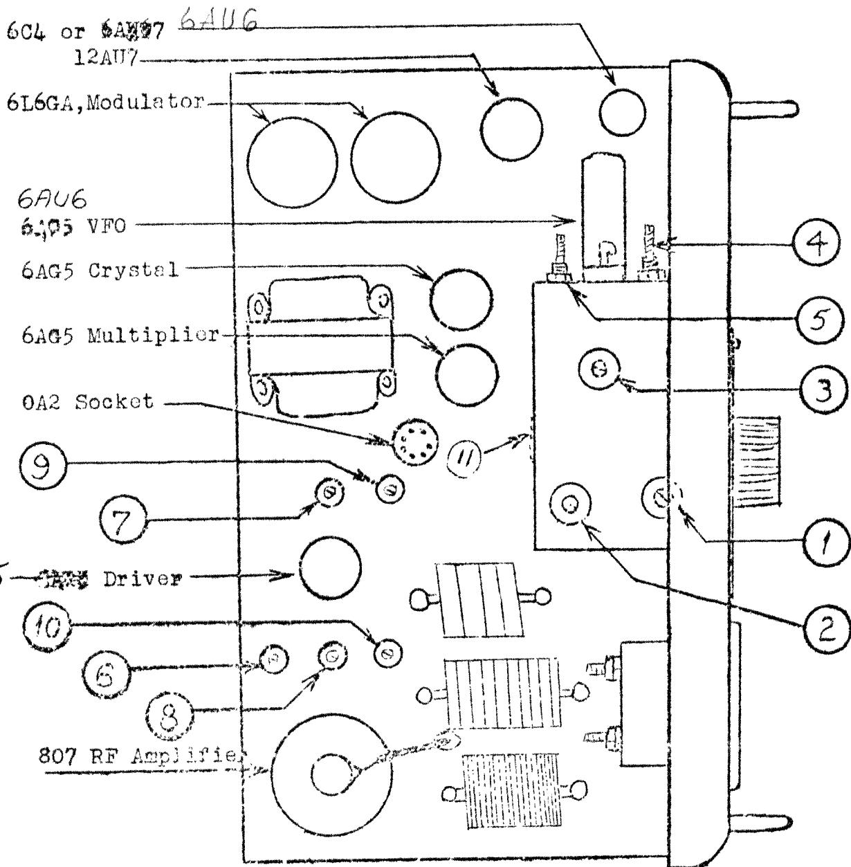
DIAGRAM showing physical layout of tubes and other component parts on the chassis of the Model A-54 and Model A-54H. The extreme top right hand tube is a 6C4 in the Model A-54 and a 6AQ57 in the Model A-54H.
