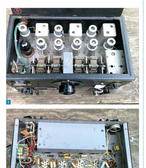
which intrinsically changes as the L/C (inductance/capacitance) ratio changes, a high-inductance primary is used in the inter-valve RF transformers, leading to the opposite, which is then compensated for by having a small top-coupling capacitor between primary and secondary. This however is not shown on the circuit diagrams.
