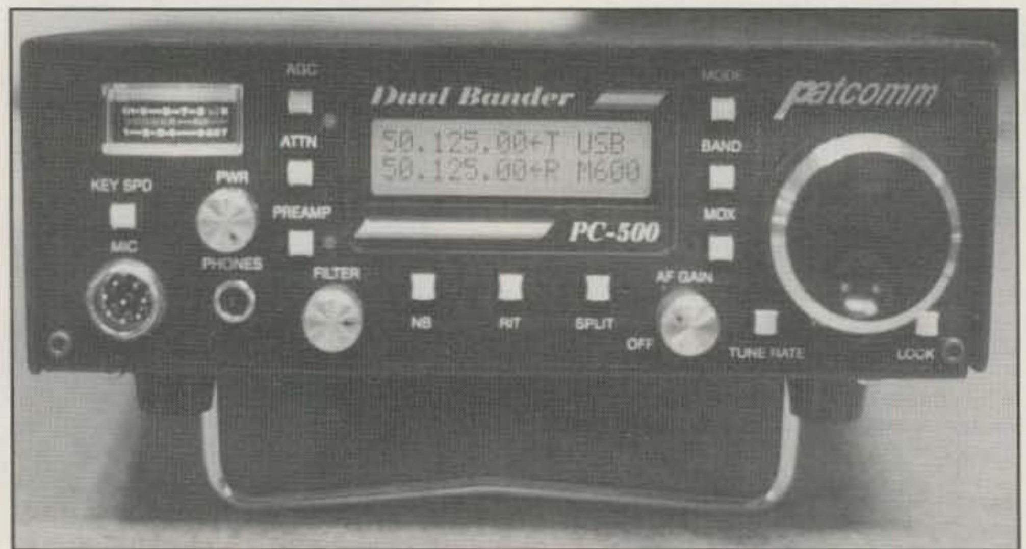
Front panel view of the PC-500 dual-band transceiver. There is a large S-meter panel on the left and a main LCD display for showing two lines of frequency, one for the receive mode and the other for the transmit mode.
