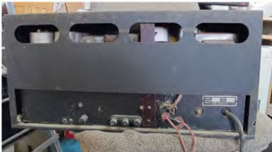
The original mains wiring in the receiver was unusable and unsafe, as shown. It was replaced with three-core cord with a chassis gland.
