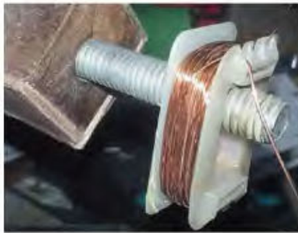
A Jaycar Cat. MM2007 transformer was rewound to act as the matching transformer for the speaker unit.
