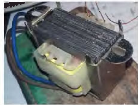
A Jaycar Cat. MM2007 transformer was rewound to act as the matching transformer for the speaker unit.
