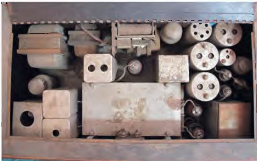
The inside of the receiver, as originally received, was full of dust and showed some surface rust.
