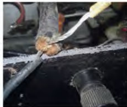
The original mains wiring in the receiver was unusable and unsafe, as shown. It was replaced with three-core cord with a chassis gland.
