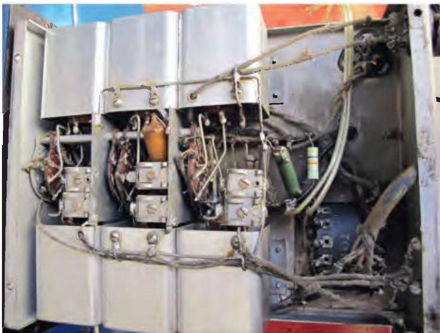
Left: the original underside of the DB-20 pre-selector. The DB-20 provides continuous coverage from 550kHz to 32MHz in six bands, and has a gain of ~20-25dB which is the basis for its name. The DB-20 was also used by the US Navy under the name CME-50063.
