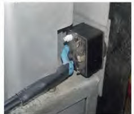
Below: a replacement switch for gain control "A" on the front panel.
