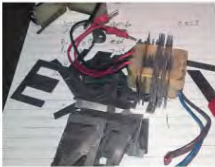
A Jaycar Cat. MM2007 transformer was rewound to act as the matching transformer for the speaker unit.
