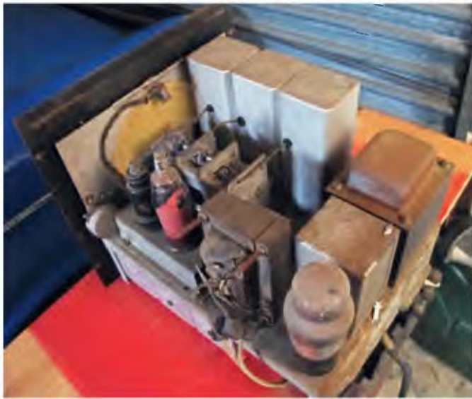
The DB-20 pre-selector had a very worn filter choke hanging off the lower left of the chassis. This choke, the power supply transformer and the type 80 rectifier valve were removed and replaced with a \pi filter.
