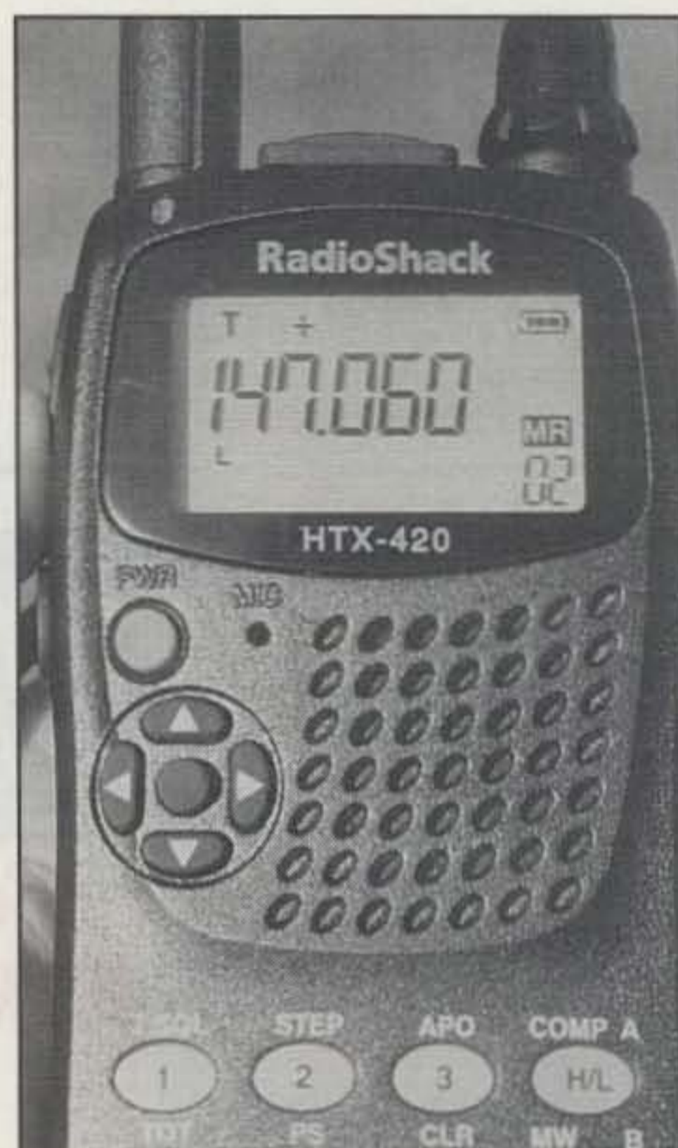
The big LCD readout on the RadioShack HTX-420 shows that the radio is tuned to 147.060 MHz, using tone and a positive shift, on low power, in memory position 2, and that the battery is in good shape. (Photos by the author)
