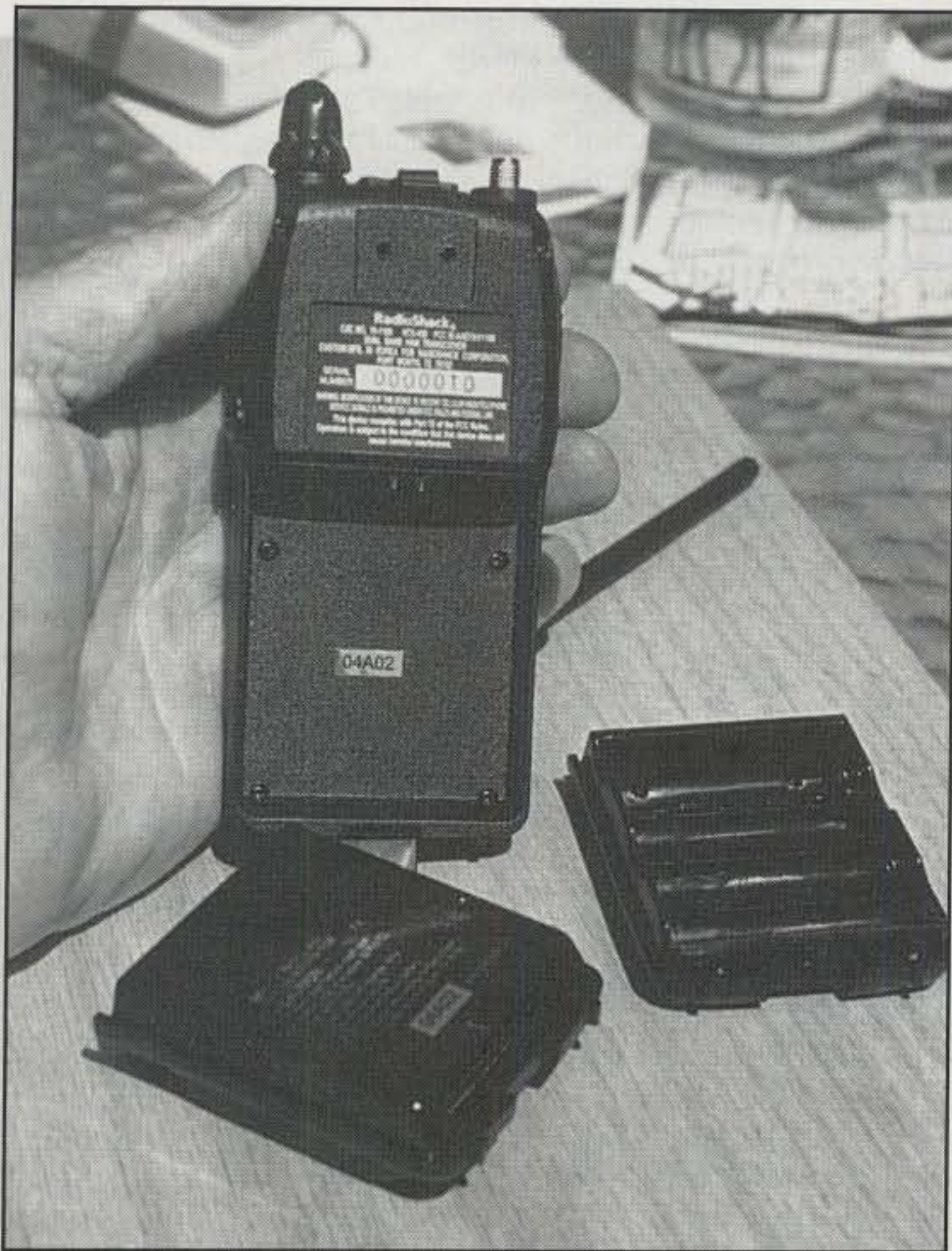
The HTX-420 comes standard with a 7.2 volt, 1200 mAh lithium ion battery pack (with wall charger), plus a holder for four AA batteries of your choice. Using an optional power cord, you may also plug into a 12 volt DC supply.
