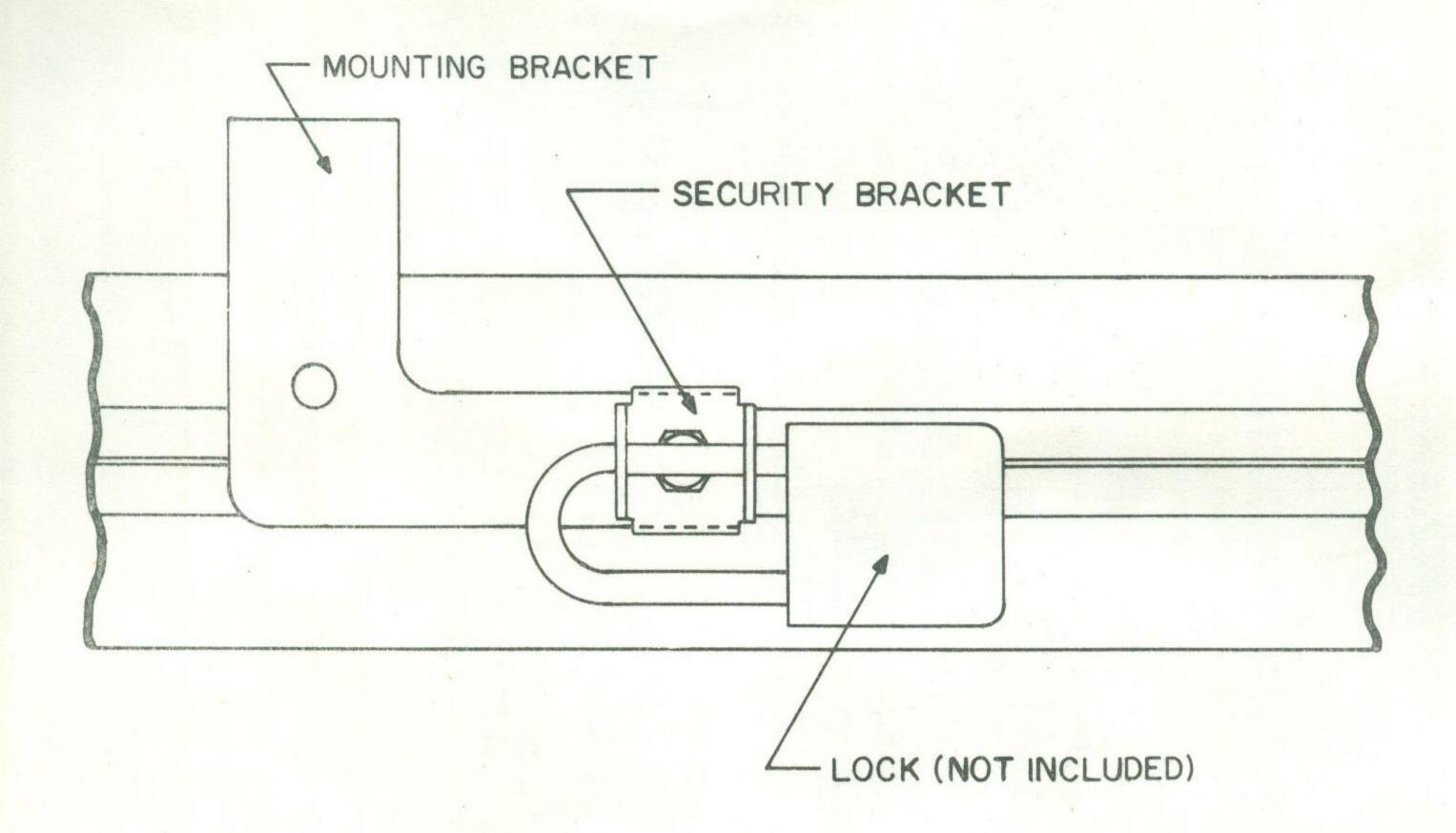
SIDE VIEW SHOWING SECURITY BRACKET INSTALLATION
