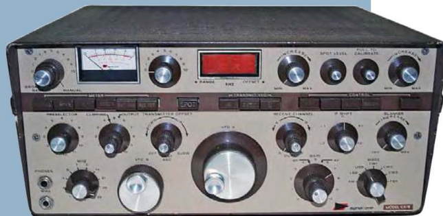
Figure 3 — A modified CX-7 from the CX-7A and CX-7B upgrades. The modified one shown incorporates the CX-7B's power supply and LED keyer and counter board. [Dennis Kidder, W6DQ, photo]
