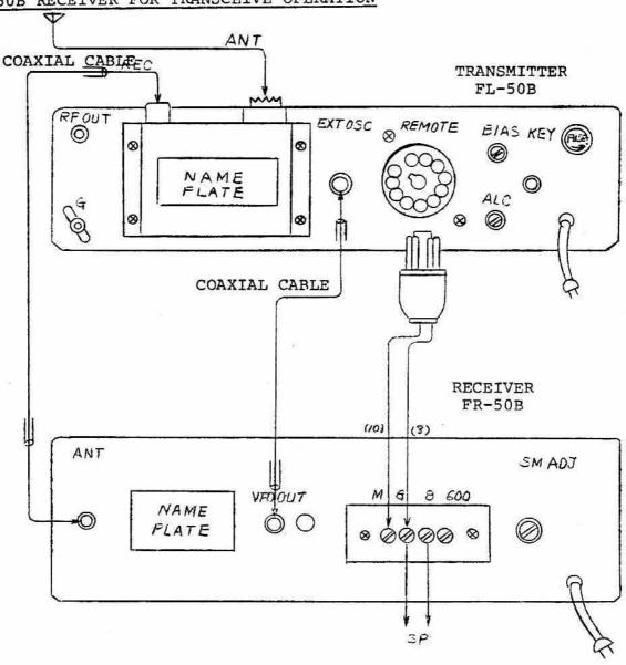
If receiver is used while disconnected from transmitter, M & G terminals must be shorted together.
