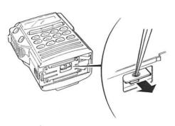
3 Attach the CMU160/CMU161 onto the transceiver. To attach, hold the CMU-160/CMU161 with the surface on which the components are not mounted facing upward and plug it straight as shown in the illustration.
