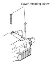
7 Attach the electrode using the screws removed in step 2.
