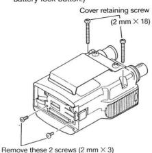
4 Place the unit with the control panel (the side from which the display can be seen) facing upward. Hold the control panel case and open it gently toward the right.
