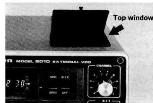
Top window for installing crystals
