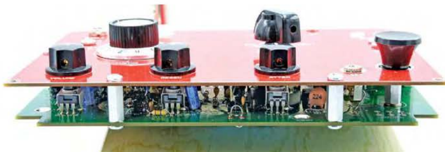
Figure 3 — The transceiver's front panel attaches to the circuit board on six metal standoffs.
