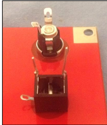
jack and plug pin arrangements
