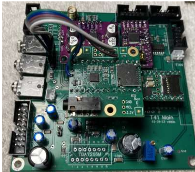
Figure 2-13. Audio board mounted on Teensy with cable.
