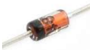
Figure 7-4. Diode with cathode marking band
