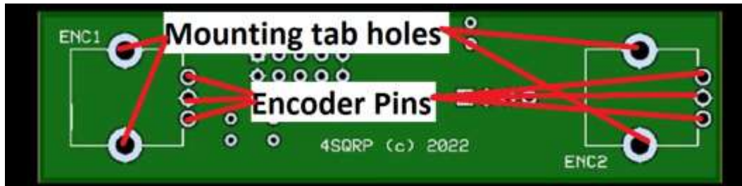
Figure 3-1. Top side of encoder PCB.
