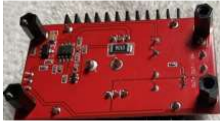
Figure 8-3. Spacer screws mounter to converter board.
