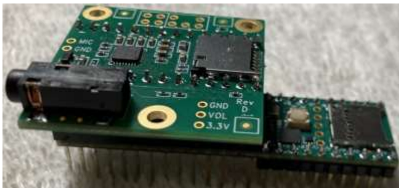
Figure 2-12. Audio board plugged into Teensy.
