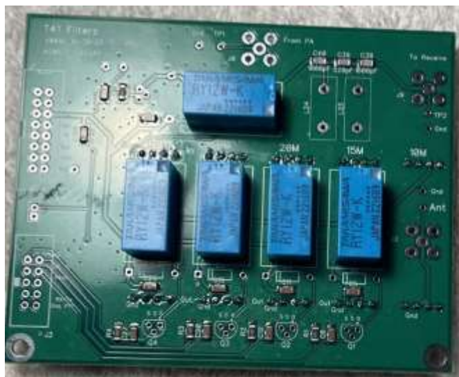
Figure 7-3. Relays mounted on main filter board.
