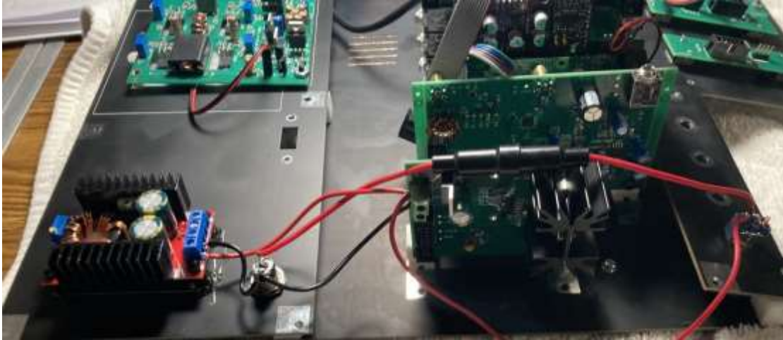
Figure 8-17. Power supply and fuse wiring.
