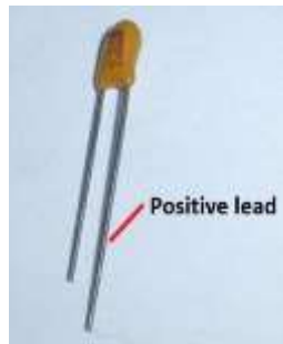
Figure 1-4. Identifying the tantalum positive lead.
