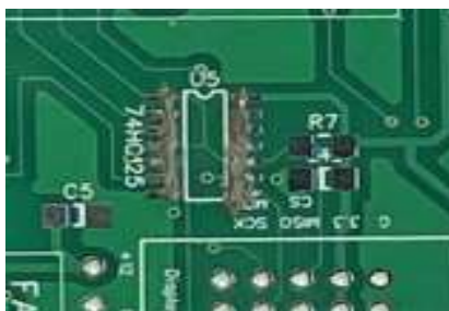
Figure Section00-1. Painting IC pins with solder paste.
