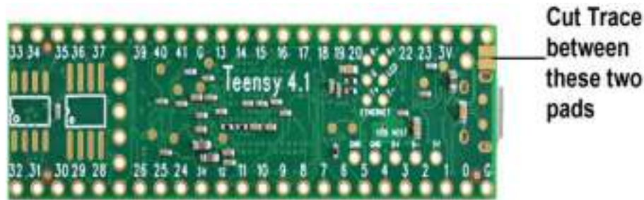
Figure 2-9. Cutting the Teensy pads.
