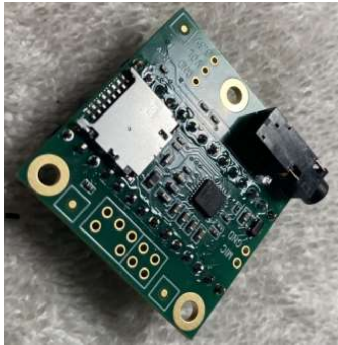
Figure 2-11. Audio Adapter Board with 2 14-pin headers solder in place.
