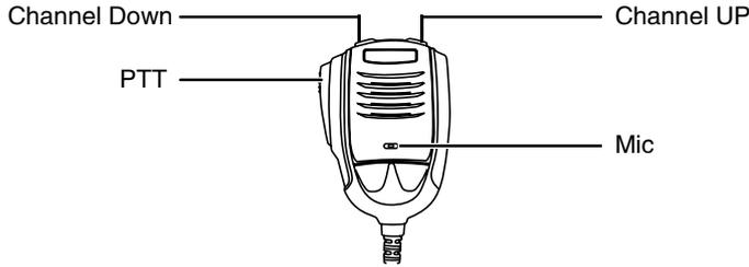
or channel through the QHM-03 microphone (Note: In professional transceiver mode, other keys are invalid except PTT, [ **UP** / **DOWN** ], [ **CALL** ] and [ **SCAN** ]).
