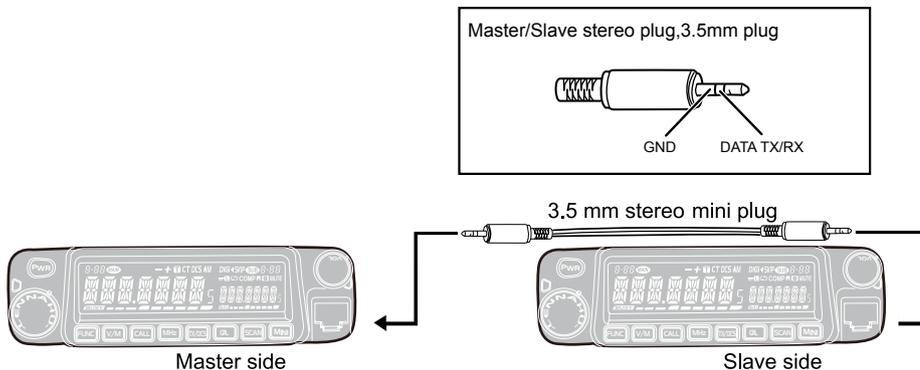
3. Press master unit's [PTT] key, LCD displays "**SD XXX**", "**XXX**" indicates data volume in transmitting. Slave unit displays "**LD XXX**", "**XXX**" indicates received data volume. When the transmission is successfully finished, the master and slave unit both display "**PASS**". Turn off the power, disconnect the cable and repeat step 2 to step 3 operations to clone the next slave unit.
