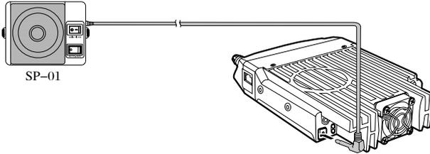
**NOTE** External speaker adopt double port BTL, please care about the connecting way. The speaker can not connect with the ground, otherwise the speaker will be fault. The wrong connecting way as the following picture.
