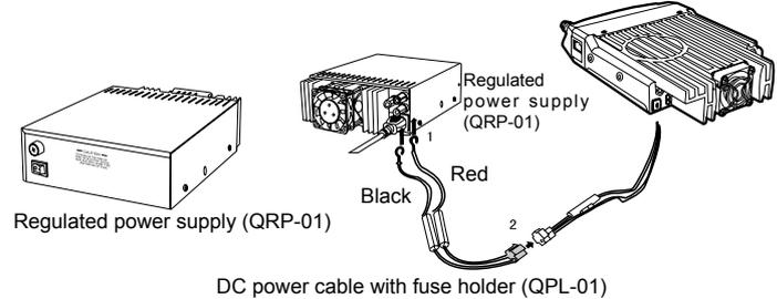
2. Connect the transceiver's DC power connector to the connector on the DC power cable.
