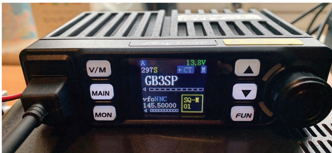
Measuring just 124mm (W) x 101mm (D) x 36mm (H) the Anytone AT-779UV is still a dual band VHF/UHF 25/10/5W transceiver.
