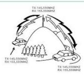
The communication between the transceiver will bread off if the repeater unable to work or the transceiver is far away the repeater which made the repeater can not transfer the signal effectively.
