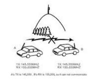
This transceiver had set a Rey to avoid this phenomenon happens. Transmitter just need to press key more than 2 seconds if you found you can not calling which caused by repeater can not provide service to reach the purpose of communication between the transceiver without repeater.
