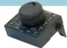
**K-Pod Controller:** Includes a precision, 400-step optical encoder for use as VFO A, VFO B, or RIT/XIT offset, plus 8 dual-function programmable switches. Can be directly connected to any K4 USB-A jack.
