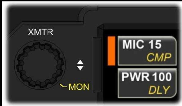
Rotate {XMTR} to adjust often-used transmit functions.
