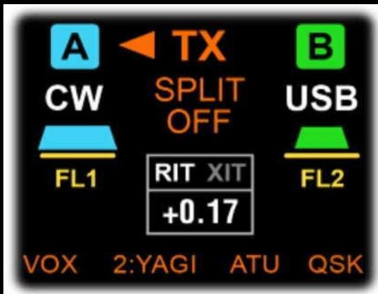
"TX" and its arrows show which VFO is selected for transmit (see [USING SPLIT](#)). The VOX icon shows that VOX is on for the current mode (see [VOX](#) switch); ATU shows whether the ATU is in-line
