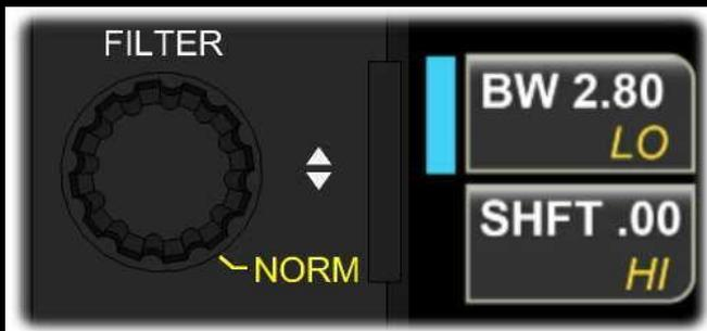
Tap the knob to alternate between <BW> (or <HI> cut) and <SHFT> (or <LO> cut). Hold the knob to select the [NORM] (normalized) passband for each mode.
