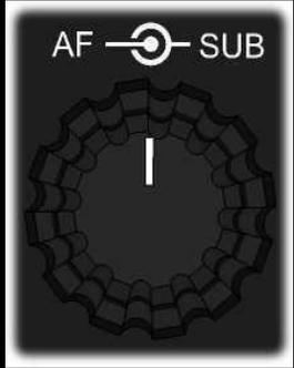
The inner concentric knob, {AF}, sets main receiver AF gain. The outer concentric knob, {SUB}, sets sub receiver AF gain.
