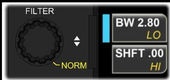
Rotate {FILTER} to adjust receiver filter bandwidth and shift, or hi-cut and lo-cut.
