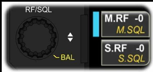
Rotate {RF/SQL} to adjust RF gain or squelch.
