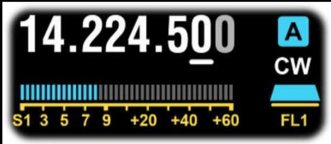
Adjacent to each VFO's numeric display is its ID (A in blue, B in green) and operating mode. Mode icons or the [MODE] switch can be tapped to change modes. See [OPERATING MODES](#) for per-mode operating instructions.
