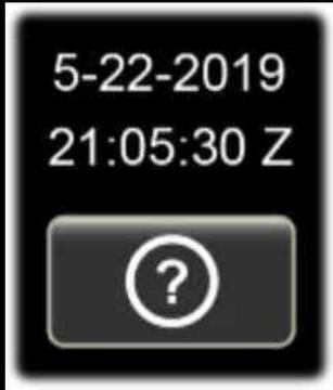
The status area, just above the Info button (<?>) at the lower-left corner of the screen, normally shows UTC date and time. Tapping this text brings up the STATUS DISPLAY button group, allowing you to select a different status display, such as your callsign and time, or supply voltage/current/power output/SWR, or main/sub signal levels in relative dB. See [USING THE STATUS DISPLAY](#) for full details.
