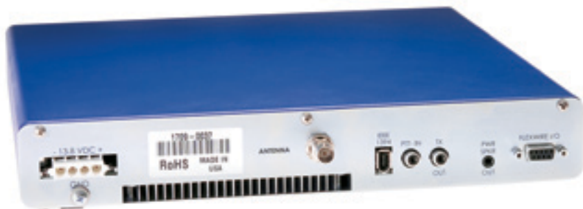
Figure 1 — Rear panel connections are straightforward — dc power, antenna, computer, amplified speakers, TR and amplifier switching and FlexWire I/O for accessories.
