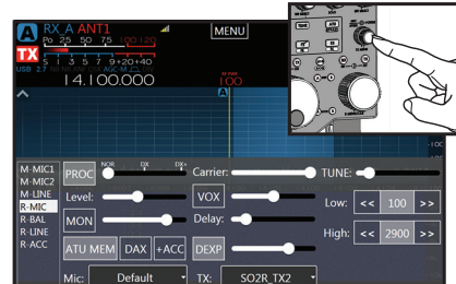
Press Power Knob for Transmit Menu
